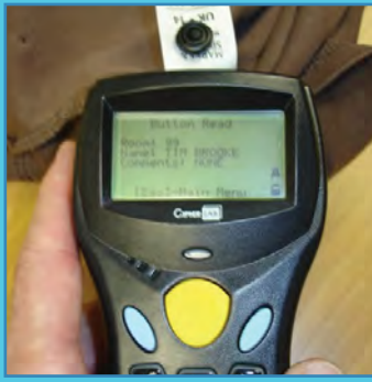
Button attached to the care label of clothing, being scanned to identify the owner
